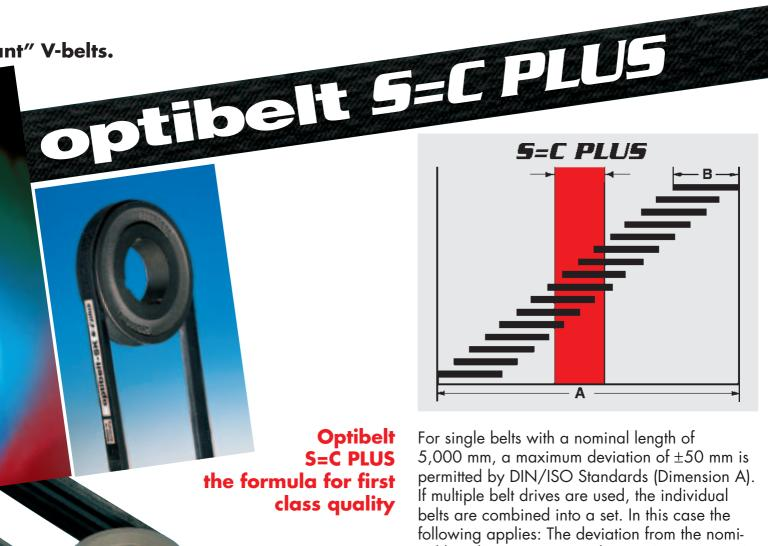
nal length must not exceed 6 mm (Dimension B). Optibelt S=C PLUS meets both requirements with ease, providing a guaranteed length tolerance of merely  $\pm 2$  mm.
